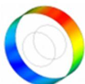
This article describes computational fluid dynamics (CFD) analysis of cooling processes of electrical Cu conductor with PVC insulation. Horizontally conductor was loaded by electric current and its cooling process was caused by influence of free convection of air and radiation. Results of CFD analysis were compared with experimental results.
