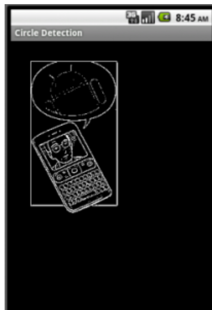
Fig. 3. Application detecting edges
