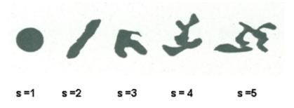
Fig.3 Pores shapes with the different roundness factor s [3]
