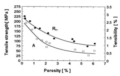
Fig.1 Influence of the porosity on the mechanical properties of the AlSiCu12 alloy.[3]
