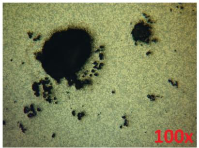
Fig.7 The microstructure of the casting (AlSiCu12) with the presence of porosity.
