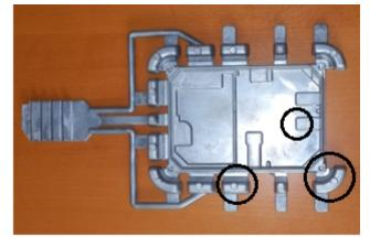
Fig.4 Choice sampling of the casting (AlSiCu12).
