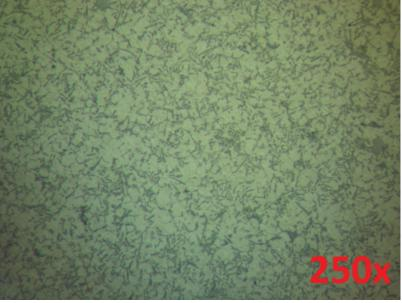
Fig.6 The microstructure of the casting (AlSiCu12).
