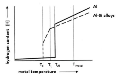
Fig.2 The effect of temperature on the solubility of hydrogen in aluminium and Al – Si alloys. [3]
