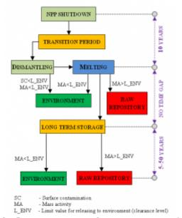
Fig. 1 The materials flow streams and time aspects of model calculation
