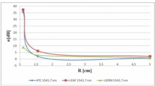
Fig.9. Dependence of attenuation on bend radius for wavelength 1541,7 nm
