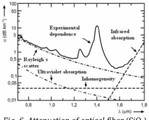
*Fig. 6. Attenuation of optical fiber* (*SiO*<sub>2</sub>)
