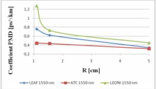
Fig.10. Dependence polarization mode dispersion on bend radius for different types of fibers
