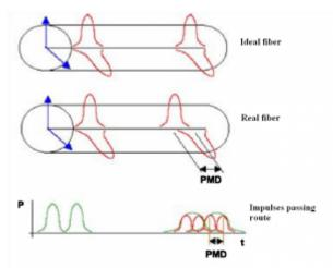
Fig. 5. Illustration of polarization mode dispersion
