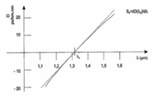
Fig.4. Spectral dependence of the chromatic dispersion coefficient D for conventional singlemode fibers,  $\lambda_0$  [nm] – wavelength of zero chromatic dispersion,  $S_0$  [ps/  $(nm^2 \times km)$ ] – slope of dispersion characteristic in area of zero chromatic dispersion
