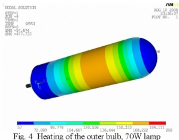
Fig. 4 Heating of the outer bulb, 70W lamp
