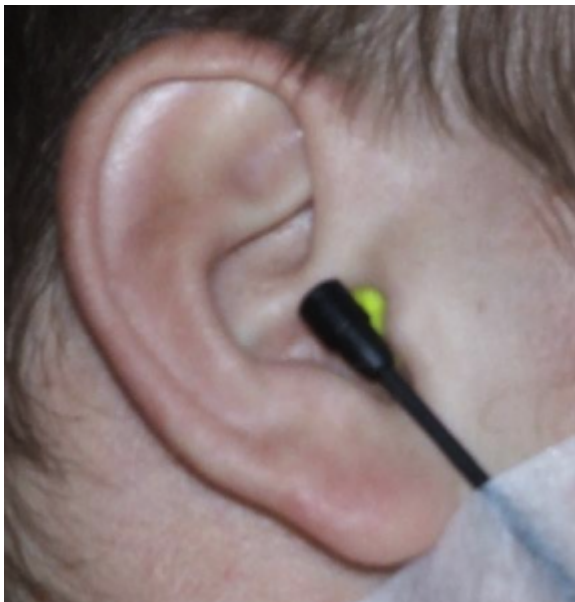
Figure 2: Measuring of HRTF - a) whole measuring set b) detail on microphone attachment.
