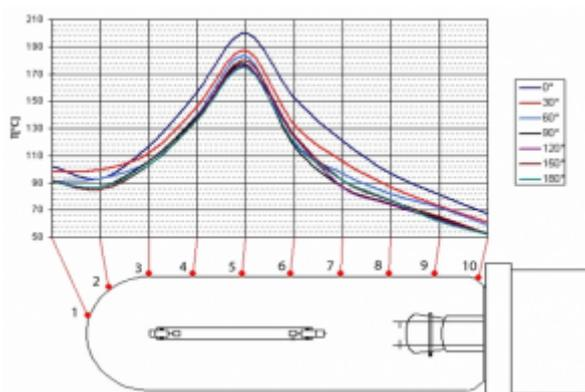
*Fig. 6 Outer heating profiles of the sodium discharge lamp 70W, radial from the top*
