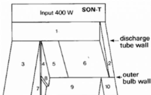
Fig. 1 Energy balance of the 400W high-pressure sodium lamp [6]
