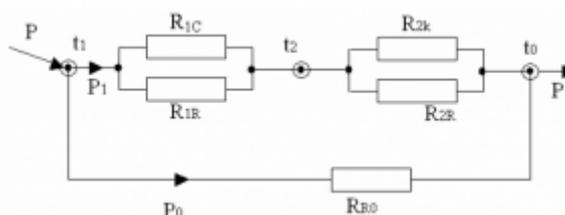
Fig. 2 Equivalent thermal diagram of the sodium discharge lamp
