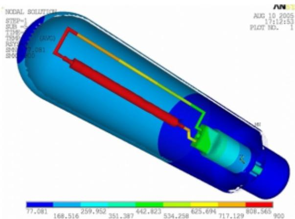
The average temperature of the outer bulb range about 120°C. The temperatures of the sides of the bulb stand between 50 and 90 °C and the maximum temperature of the bulb near the discharge tube is about 180°C. Temperature field of interior of the lamp (Fig. 5) shows the thermal stress of the consequent parts.
